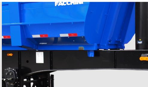
LONGARINAS VIGAS PERFIL I EM AÇO DE ALTA RESISTÊNCIA MECÂNICA, COM TRAVESSAS PERFIL U INTERLIGANDO AS LONGARINAS.
