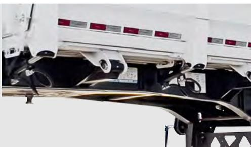
LONGARINAS VIGAS PERFIL I EM AÇO DE ALTA RESISTÊNCIA MECÂNICA, TRAVESSAS PERFIL U INTERLIGANDO AS LONGARINAS.
