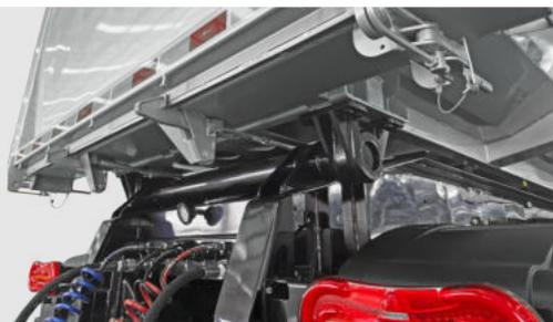
LONGARINAS VIGAS PERFIL I EM AÇO DE ALTA RESISTÊNCIA MECÂNICA, COM TRAVESSAS PERFIL U INTERLIGANDO AS LONGARINAS. ENGATE TRASEIRO MODELO ESFÉRICO
