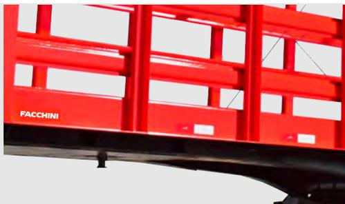
CHASSI COM LONGARINAS VIGAS PERFIL I EM AÇO DE ALTA RESISTÊNCIA MECÂNICA, COM TRAVESSAS PASSANTES PERFIL U INTERLIGANDO LONGARINAS E CORRIMÃOS EM PERFIL LATERAL Z EM AÇO LNE 38 4,5 MM.
