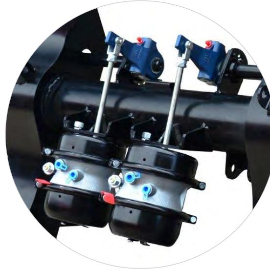
FREIO A AR, COM ABS, LINHAS DE SERVIÇO E DE EMERGÊNCIA, COM TAMBOR 16 1/2" x 8" E CÂMARA DE FREIO 30 POL<sup>2</sup> COM *SPRING BRAKE* | RESOLUÇÃO 915|22 CONTRAN
