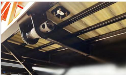
CHASSI COM LONGARINAS VIGAS PERFIL I EM AÇO DE ALTA RESISTÊNCIA MECÂNICA, COM TRAVESSAS PASSANTES PERFIL U INTERLIGANDO LONGARINAS COM SOLDA ROBOTIZADA E CORRIMÃOS PERFIL LATERAL Z EM AÇO LNE 38 4,5 MM.
