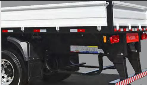
LONGARINAS VIGAS PERFIL I EM AÇO DE ALTA RESISTÊNCIA MECÂNICA, TRAVESSAS PASSANTES PERFIL U EM AÇO ASTM A36 INTERLIGANDO AS LONGARINAS COM SOLDA ROBOTIZADA E CORRIMÃOS PERFIL LATERAL U EM AÇO ASTM A36
