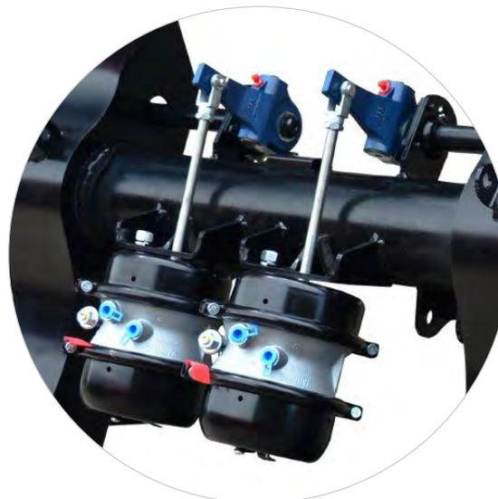
FREIO A AR, COM ABS, LINHAS DE SERVIÇO E EMERGÊNCIA, COM TAMBOR 16 ½" x 8" E CÂMARA DE FREIO 30 POL<sup>2</sup> COM *SPRING BRAKE* | RESOLUÇÃO 915|22 CONTRAN
