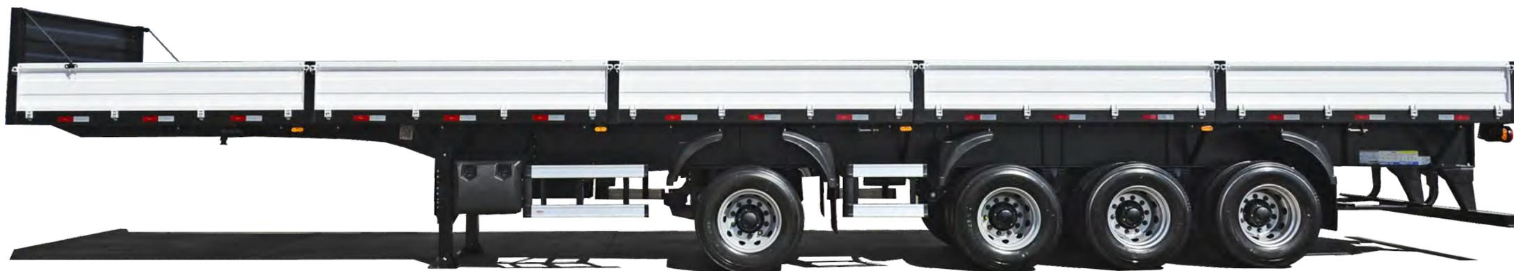
SEMIRREBOQUE COM BASE EM AÇO DE ALTA RESISTÊNCIA MECÂNICA, CONFERINDO AO CHASSI, TRAVESSAS ESTAMPADAS E PASSANTES ASA DELTA UMA ESTRUTURA QUE ALIA RESISTÊNCIA E LEVEZA
