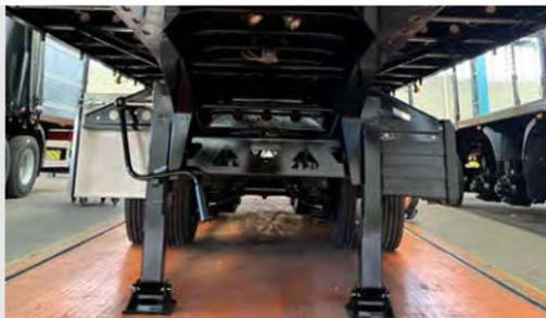
LONGARINAS VIGAS PERFIL I EM AÇO DE ALTA RESISTÊNCIA MECÂNICA, TRAVESSAS PASSANTES PERFIL C EM AÇO ASTM A36 INTERLIGANDO AS LONGARINAS POR SOLDA ROBOTIZADA E CORRIMÃOS PERFIL LATERAL C EM AÇO LNE 38
